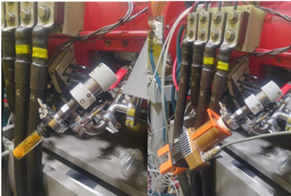
FIG. 1. The MIVOC fixture setup on the side of ECR2. The left picture shows the Ferrocene in the glass vial connected to the EVN 16 dosing valve, which is then connected to the ion source. The right picture shows the Peltier cooler installed, encasing the glass vial in the complete setup.
